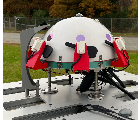
Figure 1. Left: Mechanical design drawing of the Dalek IR camera array. Right: photograph of the Dalek as constructed at the development site.
