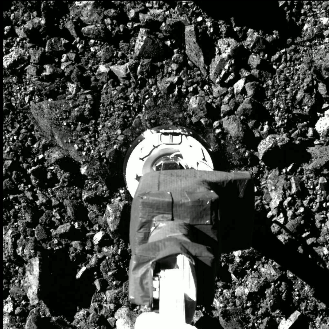
OSIRIS-Rex sample collection at Asteroid Bennu: SamCam View (NASA, Oct. 20, 2020)
