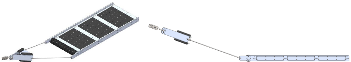
Figure 1: Magnetic sled design. Left: Isometric view of the magnetic sled design, Right: Side view of the sled when placed on the ocean floor. The 250-kg, 1-by-2-meter sled was covered with an array of 300 neodymium magnets on both sides and equipped with video cameras in the metal tow-halter ahead of it, which was anchored by a synthetic cable to a winch on the ship, the M/V Silver Star.
